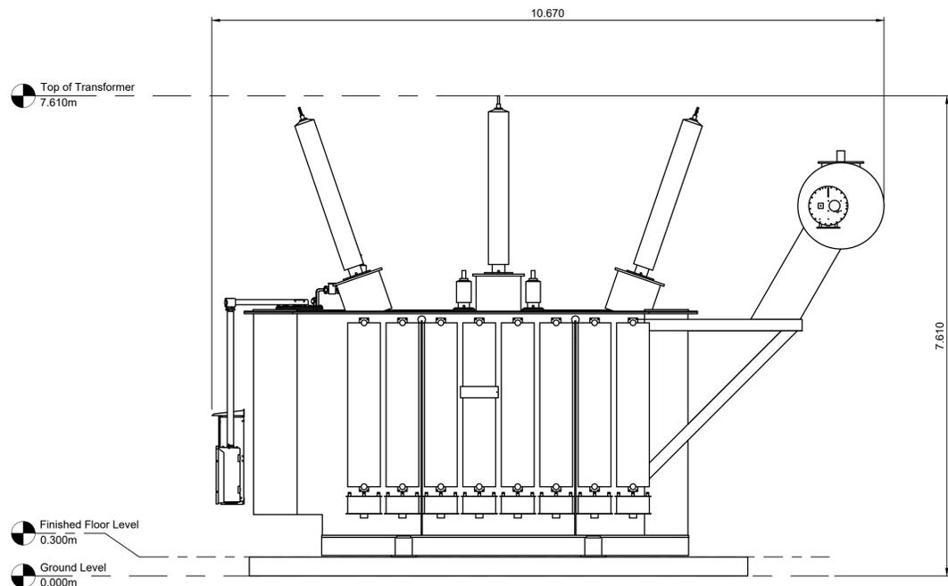
2 High Voltage Transformer South Elevation
