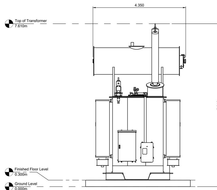
3 High Voltage Transformer West Elevation
